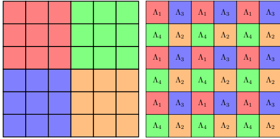
(a) Independent macro-block model: every non-overlapping macro-block of a given size is considered to be independent with the others. In this figure, the chosen size is 24 \times 24 , hence every block is only dependent with blocks with which it shares its color. (b) Lattice model: every overlapping macro-block of a given size is considered to be independent with its direct neighboring blocks. This induces four sets of blocks, called lattices, where each block in a given set is dependent with blocks in the same set.
