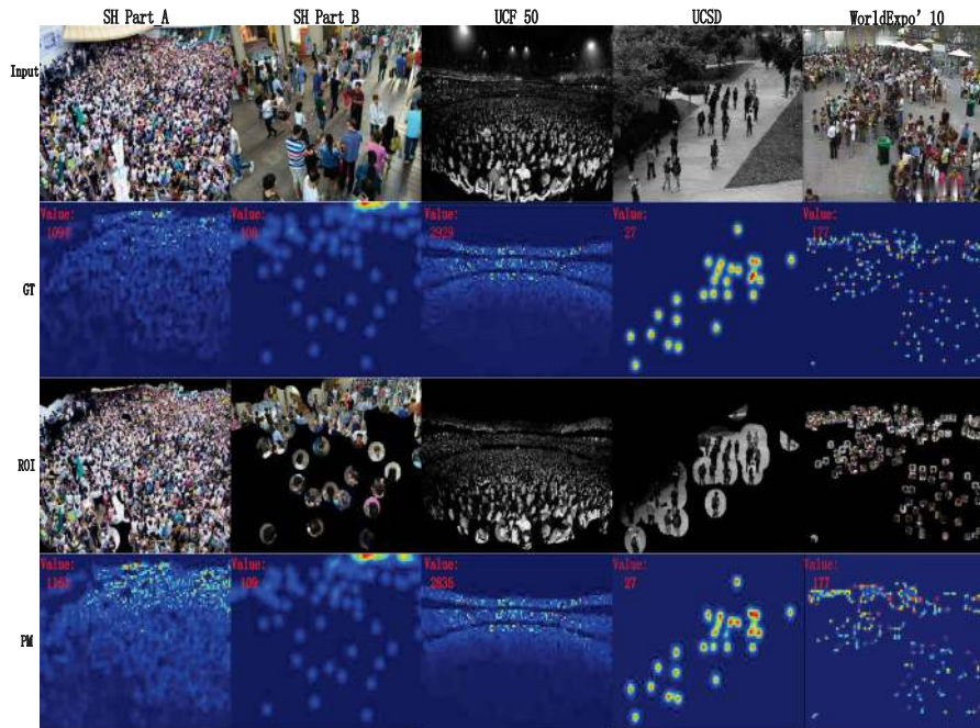
Fig. 4. The results of Dense Attentional Dilated Block Network. The attention map on five datasets. The first row shows five sample images from ShanghaiTech Part_A, ShanghaiTech Part_B, The WorldExpo'10, The UCSD, The UCF_CC_50 datasets. The second row shows ground truths (GTs) originating from datasets. The next row shows the regions of interest (ROI) multiplying input images and corresponding attention maps. The last row shows predicted maps (PMs) outputting from CDADNet.
