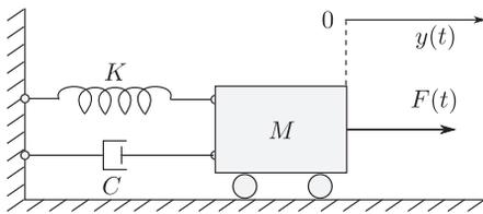
Fig. 1. Mass-spring-damper system
