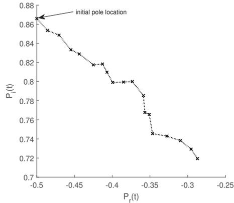
Fig. 3. Evolution of the system pole in s-plane
