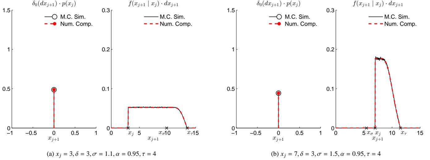
Figure 4: Shapes of the transition pdf  $P(x_j, dx_{j+1})$
