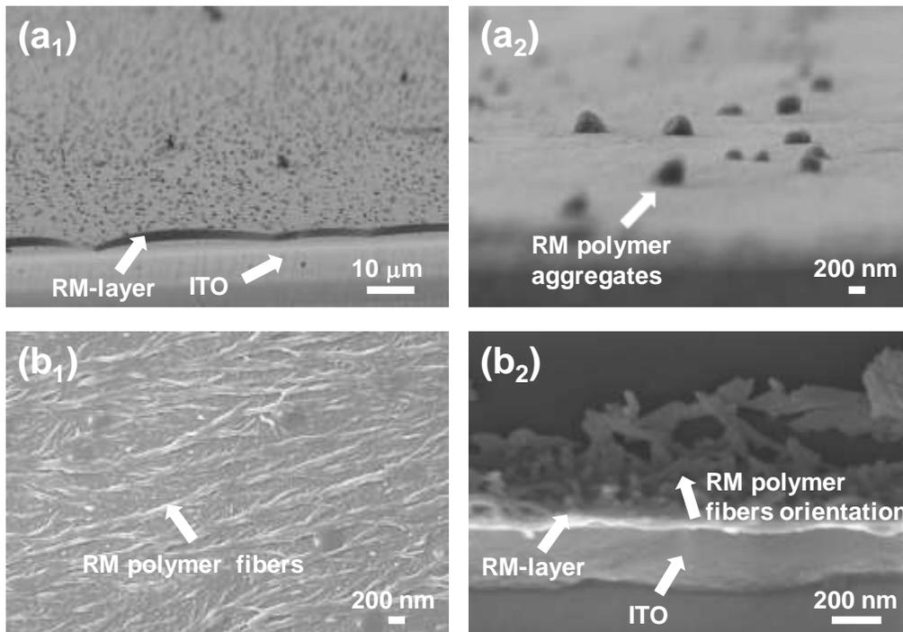
**Figure 4.** Low- (a<sub>1</sub>) and high-magnification (a<sub>2</sub>) cross-sectional SEM images illustrating the surface morphologies of the sample with the RM257 concentration of 0.05 wt%, which were observed with the sample stage tilted at 10°. Top (b<sub>1</sub>) and cross-sectional (b<sub>2</sub>) SEM images for the sample with the RM257 concentration of 0.1 wt%.
