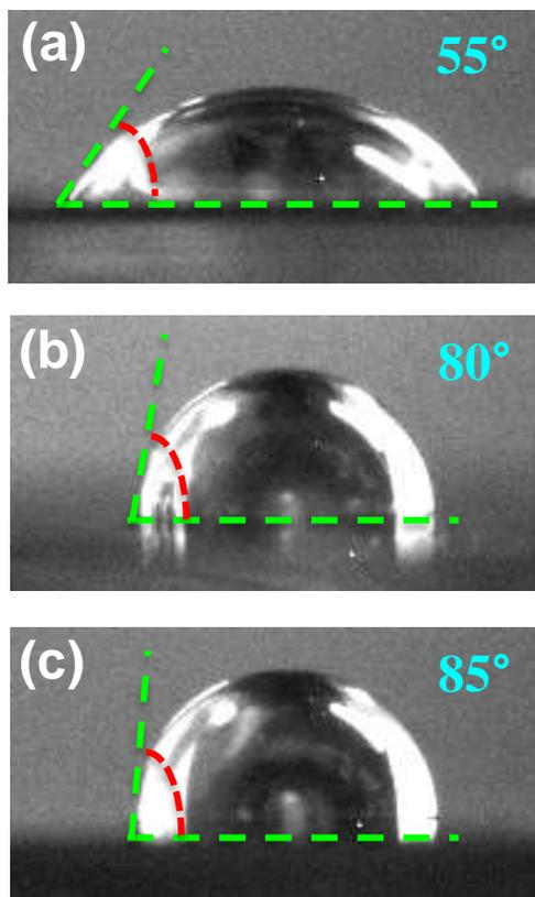
**Figure 5.** Measured contact angles for the bare ITO surface (a), RM-stabilization surfaces with low (b) and high (c) RM257 concentrations, respectively. Water with the volume of 1 mL was used as the solvent for the contact angle measurement.
