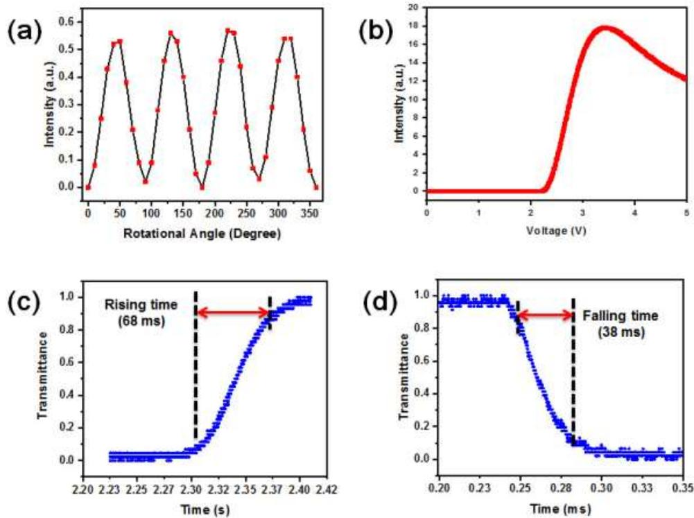
**Figure 6.** Electro-optical and switching characteristics of the LC cell after RM stabilization. (a) Sinusoidal variation of darkness and brightness at the interval of  $45^\circ$  by rotating either polarizer or analyzer. (b) Voltage-dependent transmittance curve. (c, d) Rising and falling time measurement under the driving voltage of  $3.5 V_{pp}$ .
