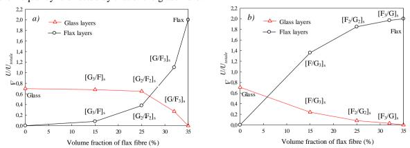
**Figure 4.** Dissipated energy in flax layers and glass layers for a 500 Hz frequency as a function of volume fraction of flax fibre in hybrid with (a) internal flax layers and (b) external flax layers.
