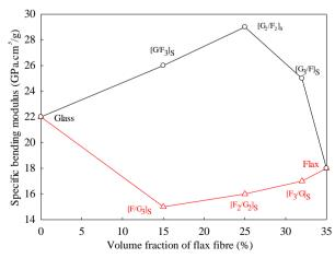
**Figure 2.** Evaluation of specific modulus as a function of the volume fraction of flax fibre of hybrid materials.
