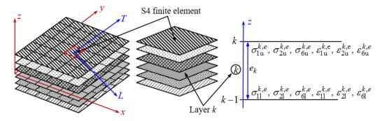
Figure 1. Multilayred finite element S4.
