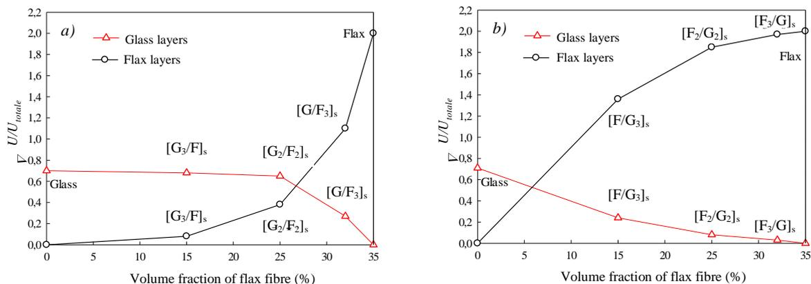
**Figure 4.** Dissipated energy in flax layers and glass layers for a 500 Hz frequency as a function of volume fraction of flax fibre in hybrid with (a) internal flax layers and (b) external flax layers.
