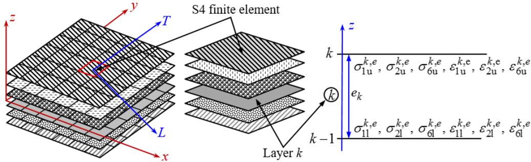
**Figure 1.** Multilayered finite element S4.
