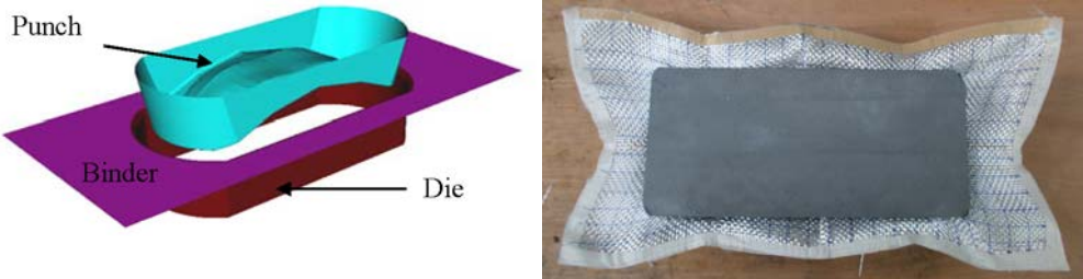
Figure 23. Experimental test of deep-drawing punch shape and final forming.
