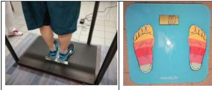
Figure 2. Left: highly standardized position of force-plate Right: standardization at home with BQT
