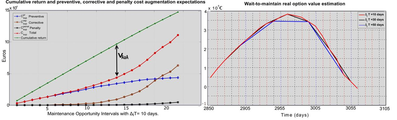
**Figure 8:** Simulation results considering changing working conditions modelled by a Markov chain: Expected values of cumulative return and the augmentation of maintenance costs between  $[t_0, t_f]$  ( $\Delta_i T = 10$  days) (Left).  $O$ : Additional gain gain in  $[t_0, t_f]$  (Right).
