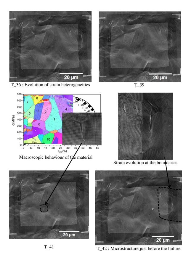
Figure 5: Strains observation on the microstructure using the displacements of the NPs on the part III of the test.
