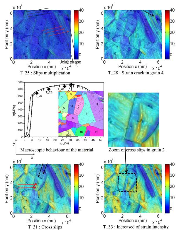
Figure 8: 2D strain maps of Part II of the test. The black arrows in grain 4 show the deformation twinnings (T\_25). The black and red arrows in grain 2 show respectively the first and second slip systems activated and form one cross slips system.
