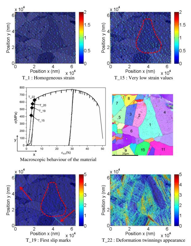
Figure 6: 2D strain maps of Part I of the test.
