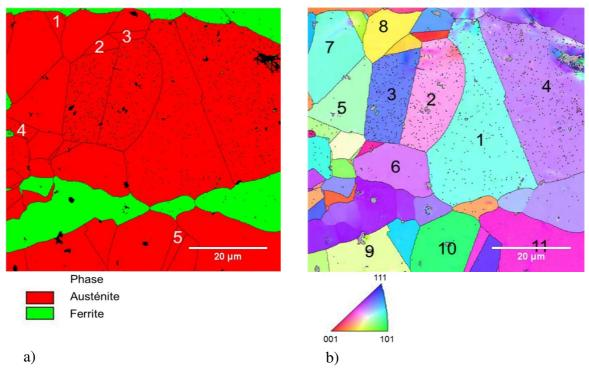
Figure 2: a) Phase distribution and b) crystallographic orientations of the microstructure component in the area of the grating.
