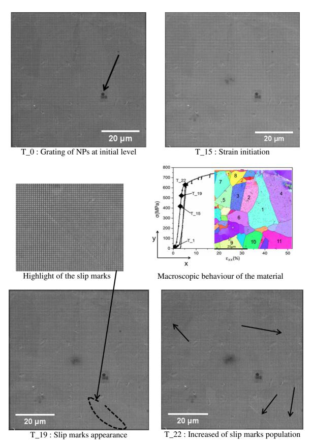
Figure 3: Strains observation on the microstructure using the displacements of the NPs on the part I of the test.
