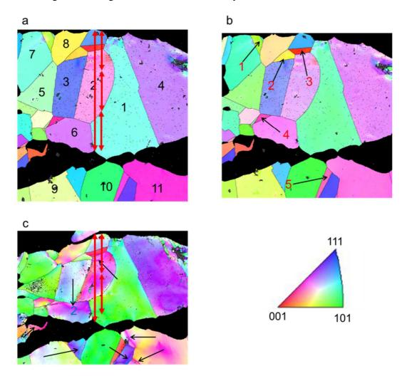
Figure 12: Inverse pole figure maps a) at the initial state, b) at the elasto-plastic transition (EBSD\_0), and c) in the plastic domain (EBSD\_1) in the austenitic phase. The numbers are assigned to grains (in black, 1 to 11) and twins (in red, 1 to 5).
