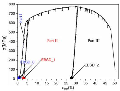
c) Stress- strain curve of the specimen with the different parts of the test.
