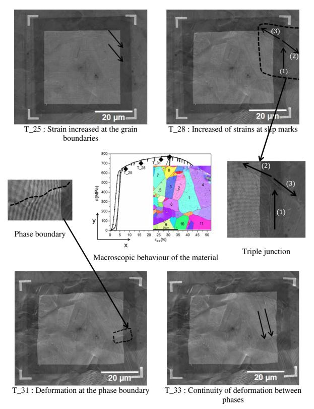
Figure 4: Strains observation on the microstructure using the displacements of the NPs on the part II of the test.
